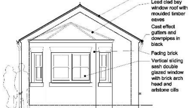
Side South Facing Elevation
